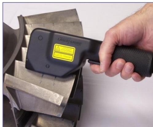
**Feedback** – Scanning is as simple as positioning the sensor on the edge of the blade and pulling the sensor trigger. Raw video and the plotted profile are displayed in real-time on the computer used with the sensor. Measurements are recorded when the trigger is released. Out-of-spec conditions are flagged with color symbols.
